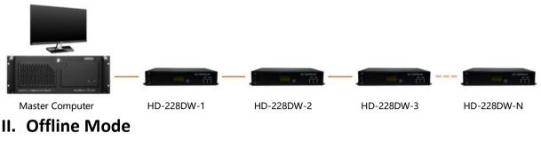
HD-228DW Connect With the Offline Master Controller, as Shown Below:
